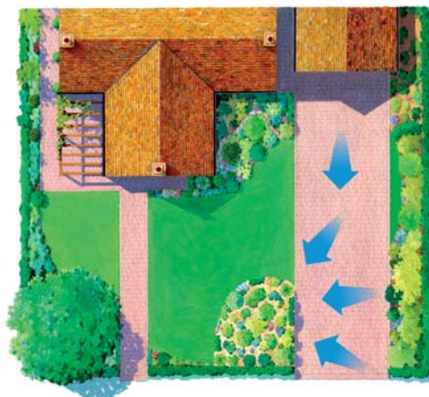
Water from conventional driveways is directed onto the rain garden
